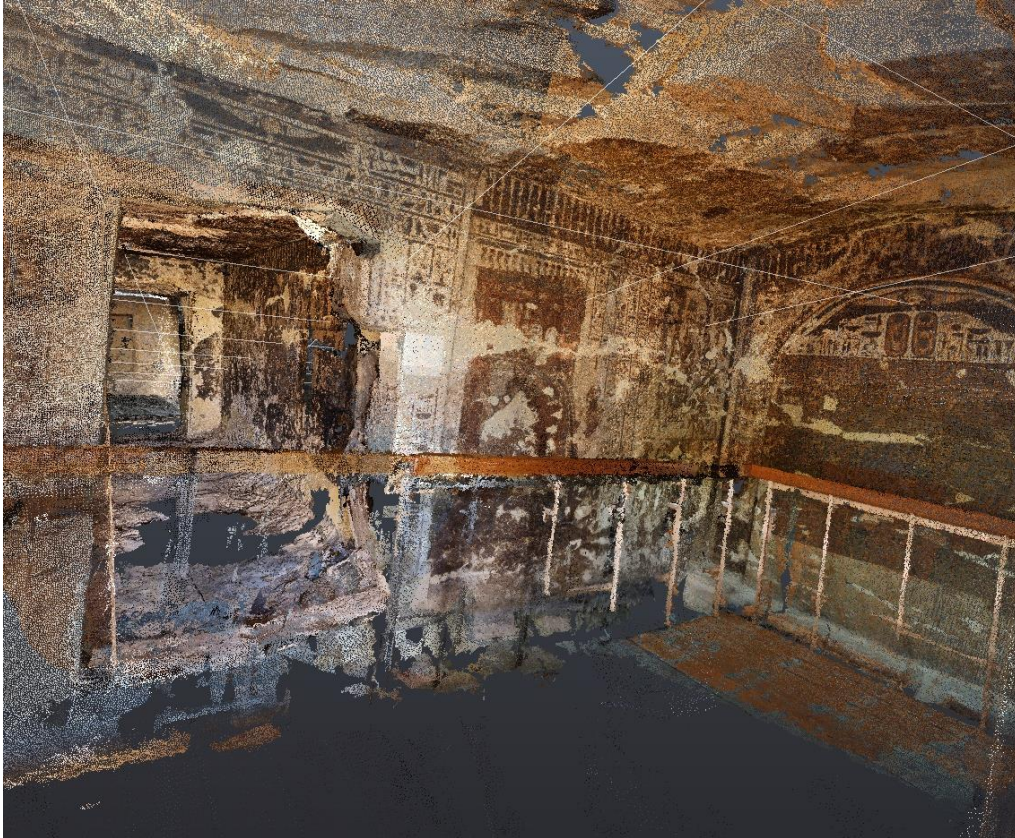
FIGURE 3: View of the dense cloud of the photogrammetric model of the tomb. Image by M. Repole.
